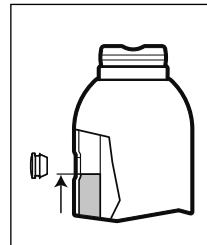
Fig. 6 - Oil Level, all models except GBJ-100
