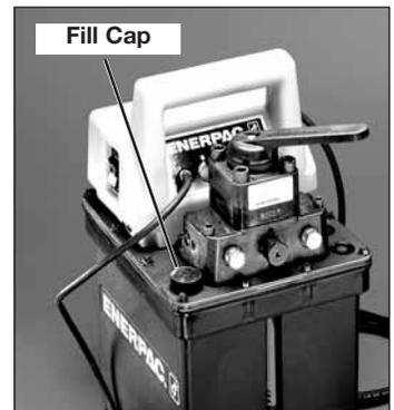
2. Check oil level prior to starting pump. Oil level gauge must be full. If required, add oil to reservoir.
