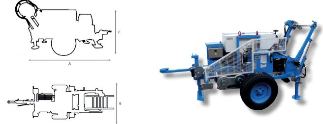
Hydraulic puller fit to pull one rope in stringing operations of overhead transmission lines. One hydraulic circuit allows to continuously vary the speed in both directions by operating one control device.
