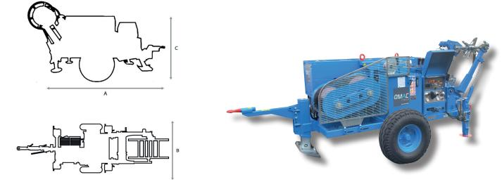
Hydraulic puller fit to pull one rope in stringing operations of overhead transmission lines. One hydraulic circuit allows to continuously vary the speed in both directions by operating one control device.
