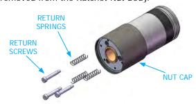
6. Having removed the Nut Cap you can then remove the upper Reaction Circlip, the Reation Plate and the lower Reaction Circlip.
