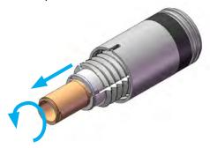
8. Having removed the collet assembly please note the centre dab marks indicating the position of the first collet section. Please also note that the collet segments are arranged on the cage such that the external ridges form one continuous thread.
