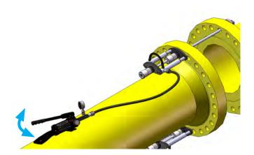
11. Continue priming the Hand Pump untill the actuators have reached full stroke 100mm (4").
