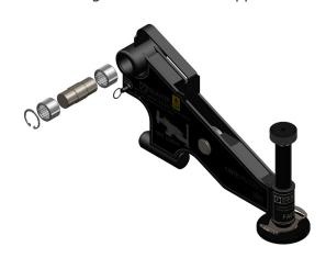
Remove the spiral retaining clips from the lower shaft and slide the shaft out from the main body.
